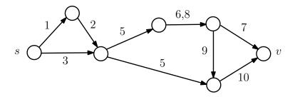
Figure 4: A violation of an invalid Menger's analogue. Both edges labeled 5 must be removed to separate s from v however there are no two out-disjoint journeys from s to v (all (s, v)-journeys must use some edge labeled 5).
